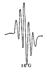
Fig. 4. EPR spectrum of the anion obtained from naphtho-1,2-selenadiazole by reduction in 1,2-dimethoxyethane using potassium metal.
